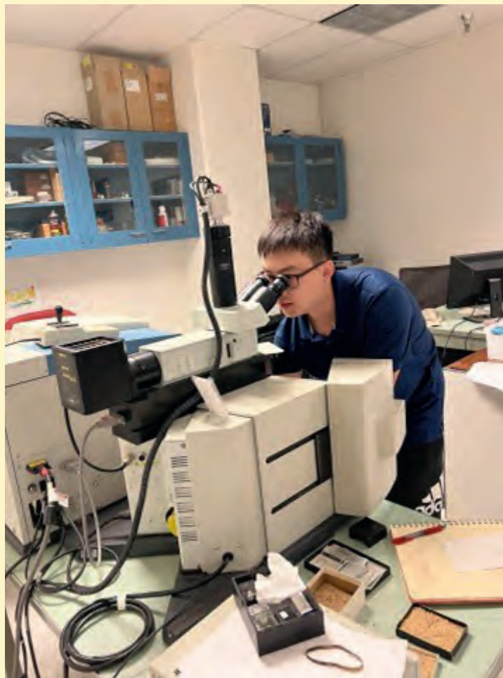
Undergraduate student Tom Zhang uses the Raman spectrometer for identifying gems and minerals
